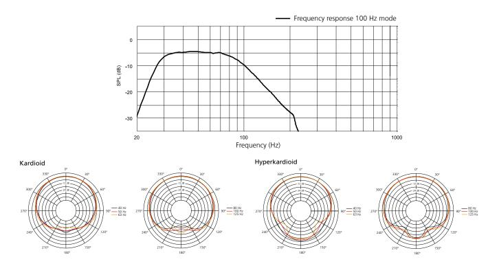
All measurements under free field conditions. Frequency patterns 1/6 octave averaged. Coverage and polar pattern 1/3 octave averaged. The manufacturer reserves the right to make product alterations to improve product quality without prior notice. Errors excepted. Attenuation factor depends on setting and configuration.
