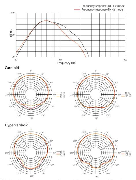
All measurements under free field conditions. Frequency patterns 1/6 octave averaged. Coverage and polar pattern 1/3 octave averaged. The manufacturer reserves the right to make product alterations to improve product quality without prior notice. Errors excepted.
