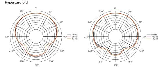
Note: Attenuation factor depends on setting and configuration (see page "Configuration and Connecting Diagramm").
