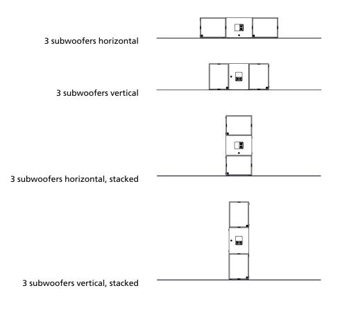
When cardioid arrays are stacked on the floor, ensure that there is always a distance of at least 40 cm between each unit of 3.
