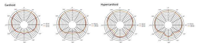
All measurements under free field conditions. Frequency patterns 1/6 octave averaged. Coverage and polar pattern 1/3 octave averaged. The manufacturer reserves the right to make product alterations to improve product quality without prior notice. Errors excepted.
