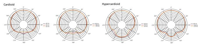
All measurements under free field conditions. Frequency patterns 1/6 octave averaged. Coverage and polar pattern 1/3 octave averaged. The manufacturer reserves the right to make product alterations to improve product quality without prior notice. Errors excepted. Attenuation factor depends on setting and configuration.
